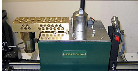
Dedicated solder pots – for lead-based or lead-free solder, each clearly marked and color-coded – prevent cross-contamination, and are quickly swappable.
