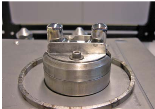
Custom nozzle with two orifices, designed to solder two connections at once.
